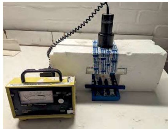
Figure 7 Monitor set-up for the radioassay calibration jig
